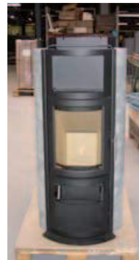
17. Both sides installed.
