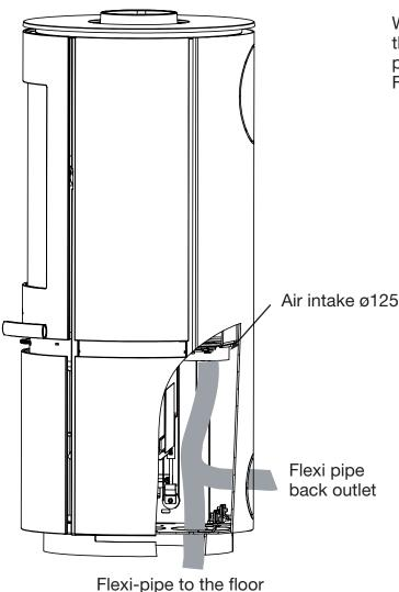
When installing external air supply, connect the air intake to the direct air pipe using flexipipe, both from the floor or behind the stove. Flexi-pipe not included.
