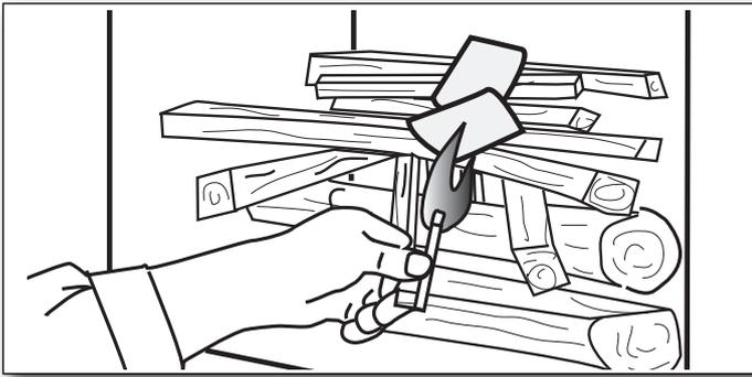
Fully open the combustion air and leave the door ajar (about 1 cm open).
