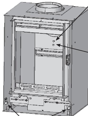
The top screw has to go through both the combustion chamber and the convection box.
